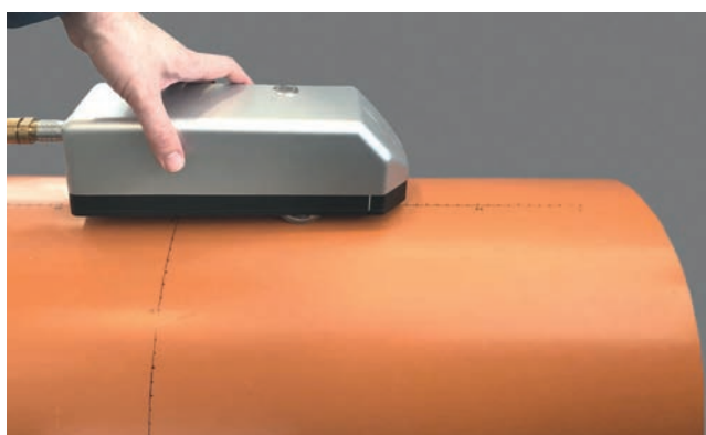
Fig. 2. Measuring setup with terahertz FMCW hand-held scanner: measurements in the field, for example on district heating pipes, are possible with the mobile terahertz sensor (© Fraunhofer ITWM)
